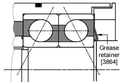
Grease retainer (clearance type) is only fitted on grease lubricated option units
