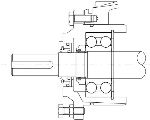
Frame 1 to 4 proprietary labyrinth/face seals (where fitted)
