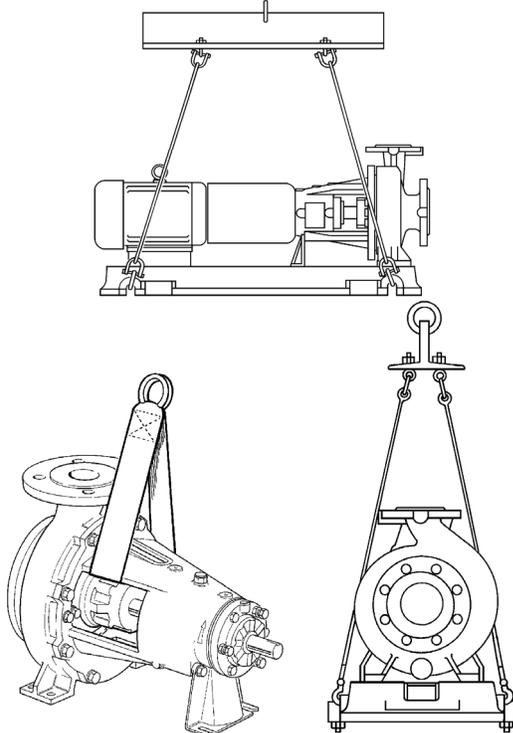
Where the baseplate is folded steel there are no specific lifting points provided for this complete machine set (unless so identified). Any lifting points that can be seen are provided only for dismantling parts for servicing. Slings, ropes and other lifting gear should be positioned where they cannot slip and where a balanced lift is obtained.
