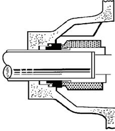
6.11.1b Single unbalanced (or inherently balanced) seal
