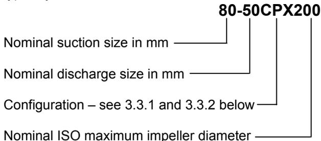
The typical nomenclature above is the general guide to the CPX configuration description. Identify the actual pump size and serial number from the pump nameplate. Check that this agrees with the applicable certification provided.
