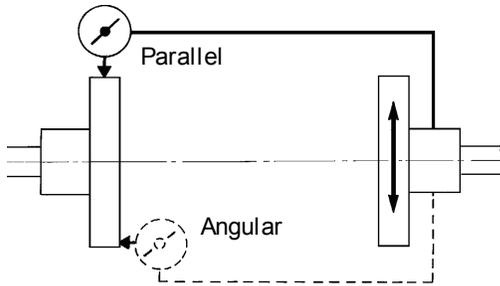
Permissible misalignment limits at working temperature:
