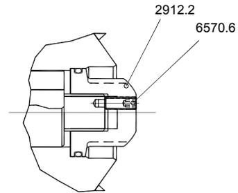
Key drive design for 304/316 stainless steel and above, secure screw with PTFE sealant (Loctite 577)
