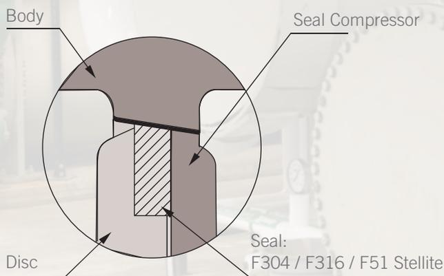
Triple offset JC valves are provided with three dimensional eccentric sealing structures. The valves are designed and manufactured with unique techniques and dedicated facilities for maximum machined accuracy. This ensures full cone match of sealing pair, and eliminates the intervention and abrasion between sealing faces.
