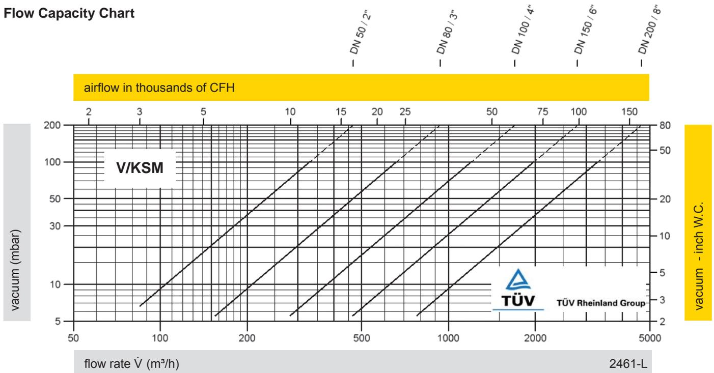
The flow capacity chart has been determined with a calibrated and TÜV certified flow capacity test rig. Volume flow  $\dot{V}$  in ( $\text{m}^3/\text{h}$ ) and CFH refer to the standard reference conditions of air ISO 6358 (20°C, 1bar). Conversion to other densities and temperatures refer to Vol. 1: "Technical Fundamentals".
