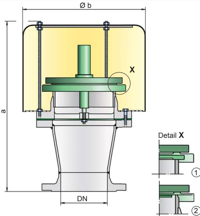
the same opening characteristic as a high pressure safety relief valve. This “full lift type” technology allows the valve to be set just 10% below the maximum allowable working pressure of the tank and still safely vent the required mass flow.
