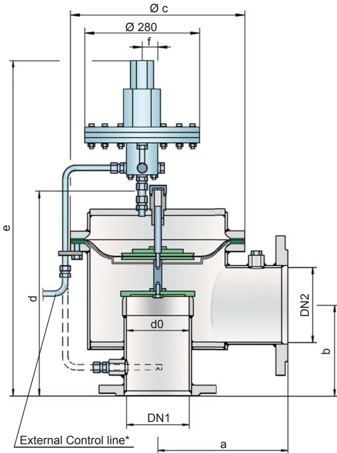
The main valve is controlled by a pilot valve. The latter in turn is controlled by the tank pressure. A small amount of fluid stored in the tank is released into the atmosphere by the pilot when the valve opens. The set-to-operate pressure is adjusted on the pilot valve by increasing or decreasing (as appropriate) the tension of a spring.
