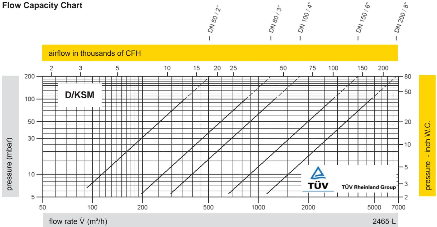
The flow capacity chart has been determined with a calibrated and TÜV certified flow capacity test rig. Volume flow  $\dot{V}$  in (m³/h) and CFH refer to the standard reference conditions of air ISO 6358 (20°C, 1bar). Conversion to other densities and temperatures refer to Vol. 1: "Technical Fundamentals".
