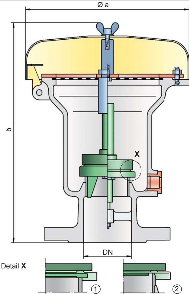
lowed PROTEGO® to develop a low pressure valve which has the same opening characteristic as a high pressure safety relief valve. This “full lift type” technology allows the valve to be set just 10% below the maximum allowable working pressure of the tank and still safely vent the required mass flow.
