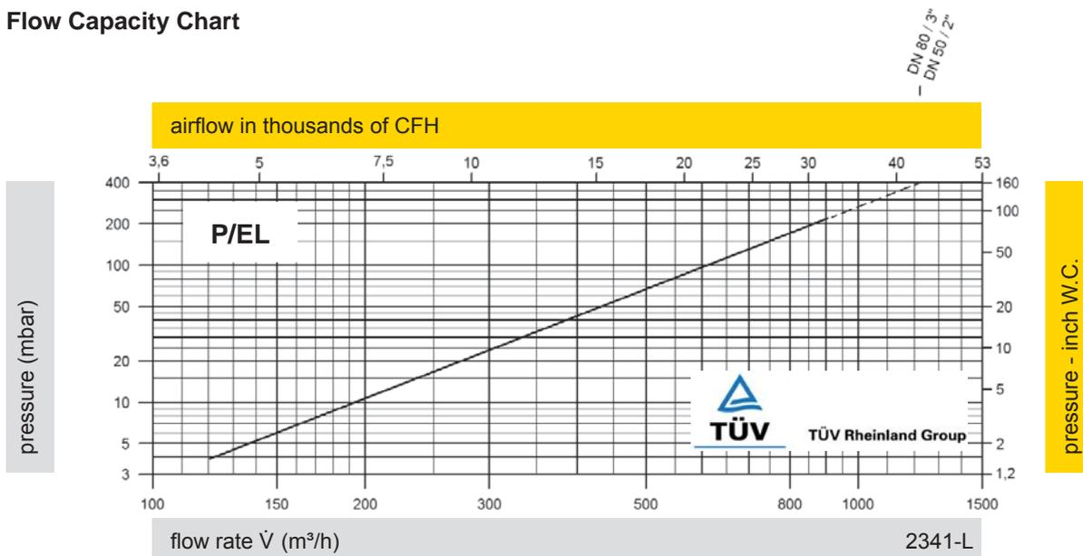
The flow capacity curve has been determined with a calibrated and TÜV certified flow capacity test rig. Volume flow  $\dot{V}$  in (m³/h) and CFH refer to the standard reference conditions of air ISO 6358 (20°C, 1bar). Conversion to other densities and temperatures refer to Vol. 1: "Technical Fundamentals".
