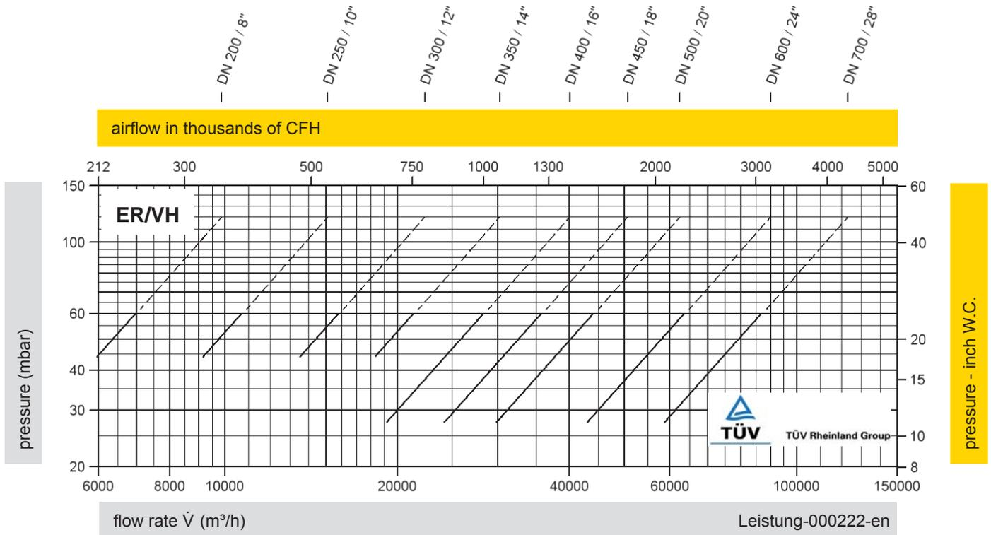
The flow capacity chart has been determined with a calibrated and TÜV certified flow capacity test rig. Volume flow  $\dot{V}$  in (m³/h) and CFH refer to the standard reference conditions of air ISO 6358 (20°C, 1bar). Conversion to other densities and temperatures refer to Vol. 1: "Technical Fundamentals".
