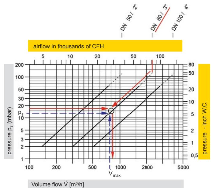
The required set pressure (= start of opening) will be the opening pressure (valve fully open) minus the characteristic overpressure.
