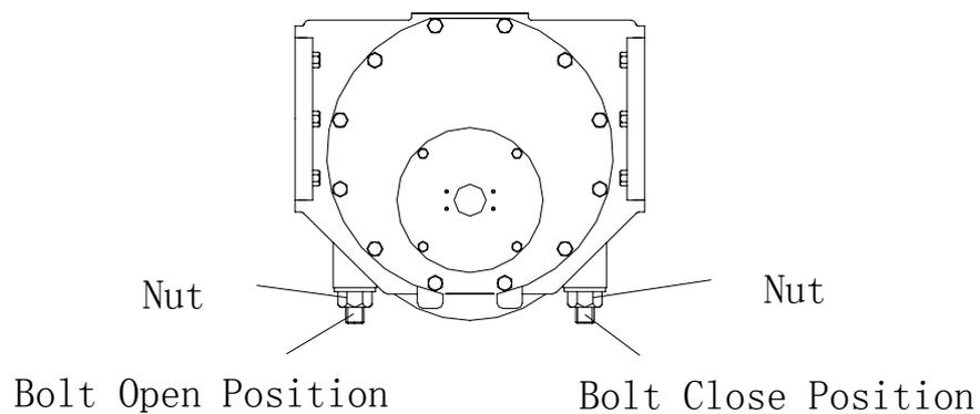
**Note:** Please note to tighten the bolt nut after adjusting the appropriate on/off position.
