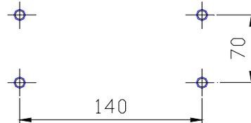
Top mounting pad of switchbox & E/P positioner
