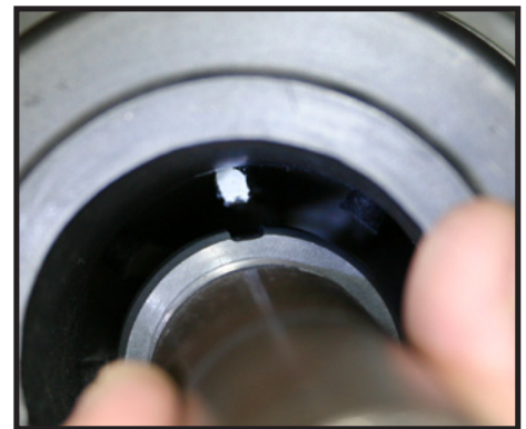
Line up the thrust control valve groove with the marked molded key.
