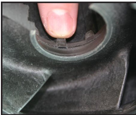
On the underside, the thrust control valve groove must line up with the molded key.
