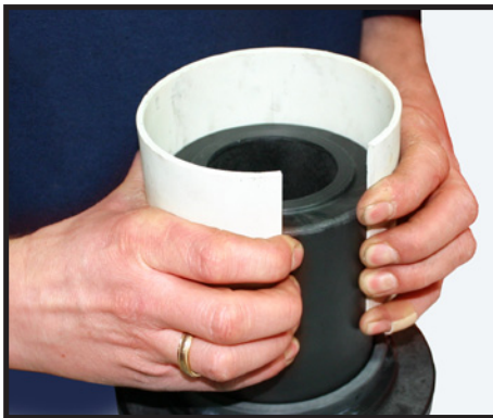
Place the trimming sleeve over the impeller to protect it from damage.
