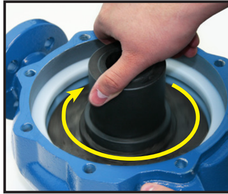
When the impeller is in place, rotate it by hand to make sure it spins freely.
