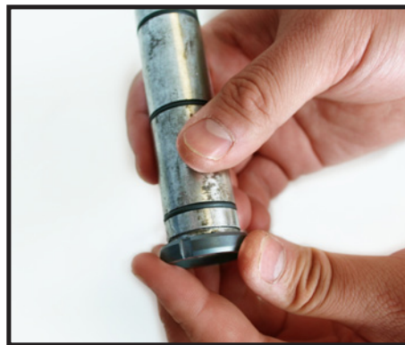
Place the thrust control valve over the rubber gasket on the stepped end of bushing installation tool part (E).
