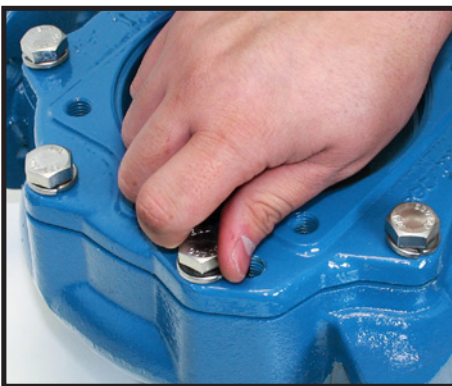
Insert and hand-tighten the (8) casing bolts with lock washers.
