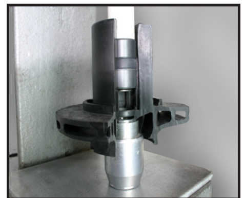
Press the bushings in until they are firmly seated using the arbor press.
