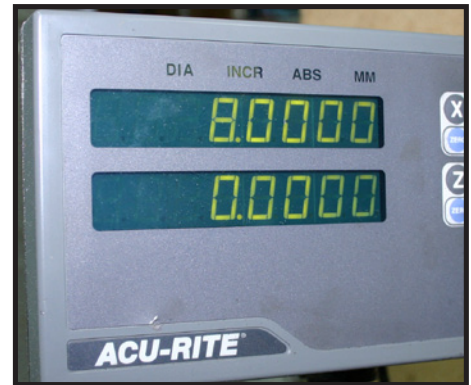
Set the trim 1/4" less then the current diameter. If you have never trimmed an impeller before, then we recommend only cutting 1/8" at a time.
