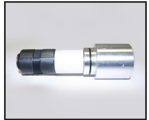
Add the white plastic spacer and the large top piece of the bushing tool.
