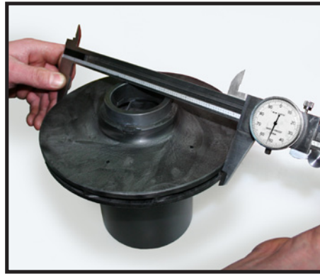
Measure the current diameter of the impeller. In this example it is 8.25"
