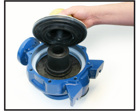
Align the shaft in the containment shell with the bushings.
