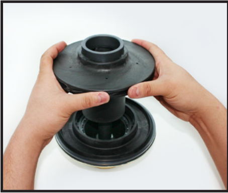
Align and slide the impeller magnet assembly onto the pump shaft located inside the containment shell.
