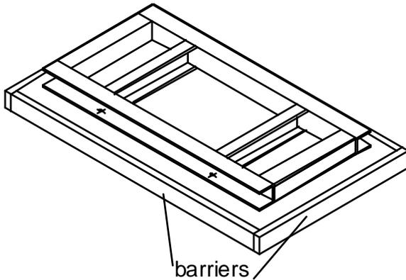
Prepare grouting product (concrete, resin) in accordance with manufacturers' instructions. (Use anti-shrink products)
