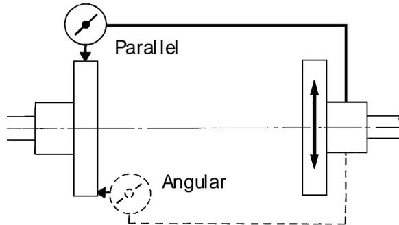
Maximum permissible misalignment at working temperature:
