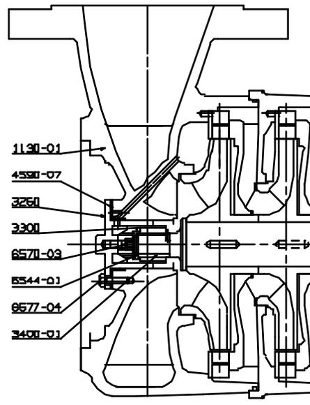
Unscrew the bearing cap screws [6577-04].
