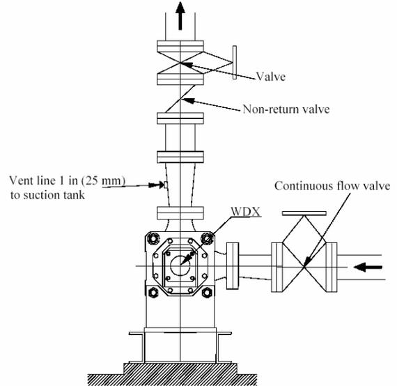
**Note:** Ideally reducers should be limited to one pipe diameter change, ie 150 mm (6 in.) to 200 mm (8 in.). Must have a maximum total angle of divergence of 15 degrees.
