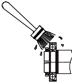
*To remove badly oxidized grease which refuses to come off:*
