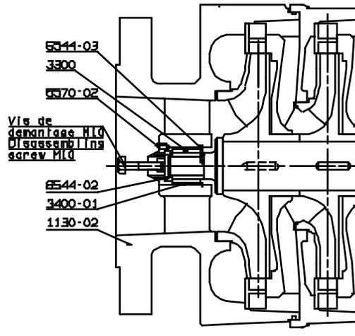
Free the bearing by removing screw [6570-02].
