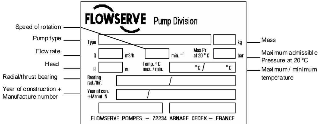
Each pump unit is supplied with the following nameplate:
