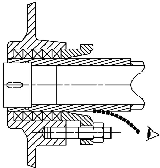
If the pump has a packed gland there must be some leakage from the gland. Gland nuts should initially be finger-tight only. Leakage should take place soon after the stuffing box is pressurized.
