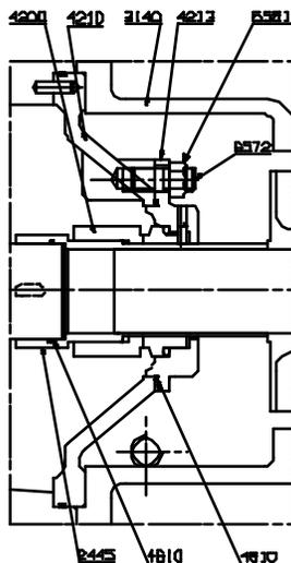
The replacement of a mechanical seal requires the dismantling of thrust and line bearing assembly. The dismantling procedure of the mechanical seal is self explanatory when viewing the respective seal drawing.
