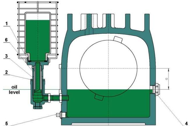
1 Denco Oiler      2 lock nut      3 adjusting sleeve
