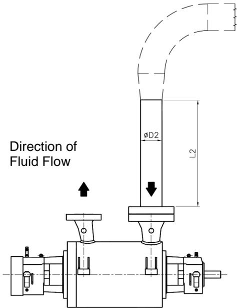
The minimum required straight pipe length (L2) before pump suction inlet is specified in Table 01. The straight pipe section is to be the same diameter as that of the pump section nozzle.
