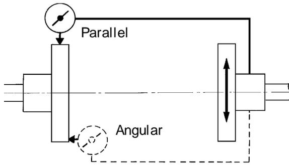
Ensure pump and driver are isolated electrically and the half couplings are disconnected. Align the motor to the pump, not the pump to the motor. Alignment of the motor is achieved by using the adjustment screws.
